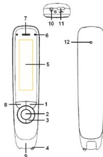
**1. Power On/Off & Back button:** A long press powers the device on or off. In the sub-interface, press this button to exit from the current level back to previous interface. When prompted for selection or input, this button cancels the operation.
