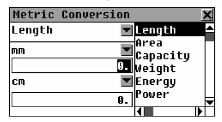
To select an option, touch its name or highlight it and press ENTER. To hide a menu without making selection, press ESC or touch the screen outside the menu area.
