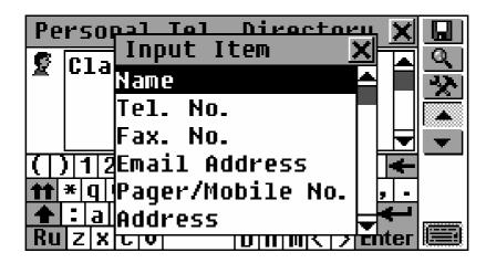
Touch a line with the stylus or move the highlight bar to a line with the arrow keys and press ENTER.
