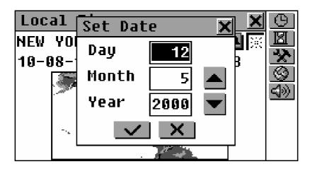
To change a value in a highlighted box, touch the buttons or press the  $\uparrow \Psi$  keys. To change the active box, touch it or use the  $\leftarrow \rightarrow$  keys. Touch or press ENTER to save settings and close the window.
