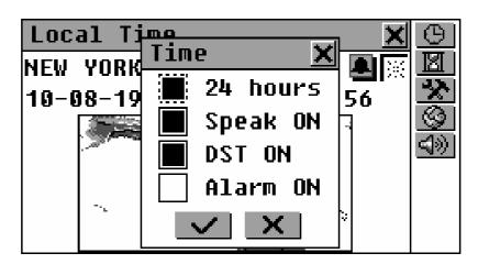
Check an empty box by touching it or by moving the dotted frame to the desired item with the arrow keys and pressing SPACE on the keyboard. A checked
