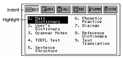
The keyboard equivalent of touching a highlightable item is moving the **highlight bar** to it with the arrow keys *and* pressing ENTER.
